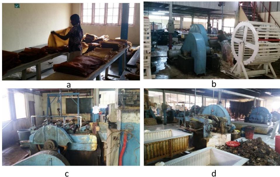
Fig. 1.2. Snapshots of a crepe rubber factory. (a) A female worker is doing visual-grading of crepe rubber, (b) A female worker operates a heavy-duty machinery called smooth roller, and (c and d) heavy-duty roller mills which require a lot of electricity, and fresh water for cleansing rubber and cooling.
