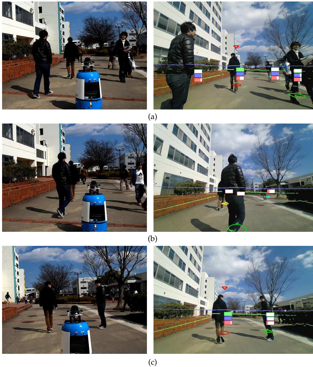
FIGURE 3.36: Specific person following experiment: The left column shows experiment scenes and the right column shows view of the camera on the robot. The meanings of the markers (triangle, circle, bars) are the same as in Fig. 3.35.
