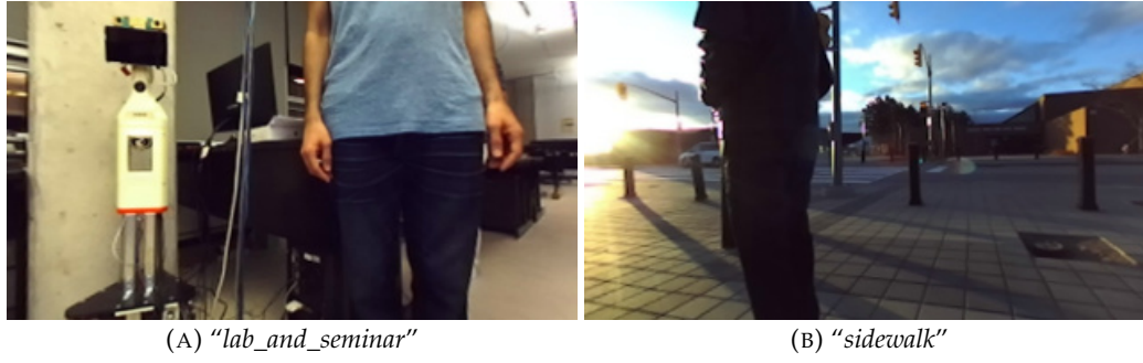
FIGURE 3.8: Failed scenes. The target person was too close to the camera, and the system failed to detect him.
