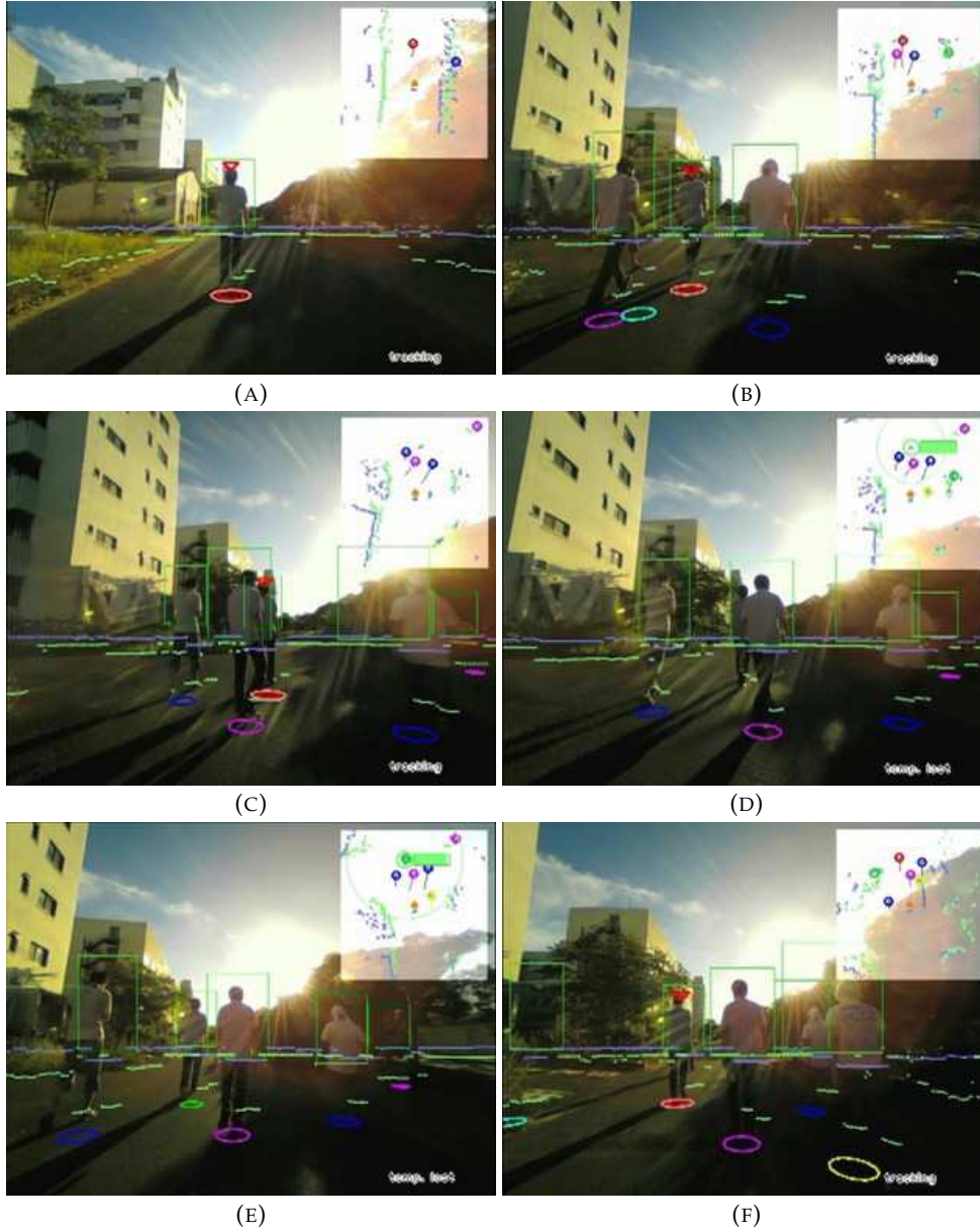
FIGURE 3.25: Person identification experiment in a severe illumination environment: Red triangles above green rectangles indicate the identified target person.
