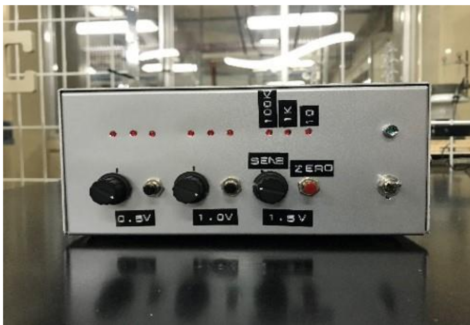
Fig. 3.29 A monitoring device for partial discharge detection front view of the monitoring device.
