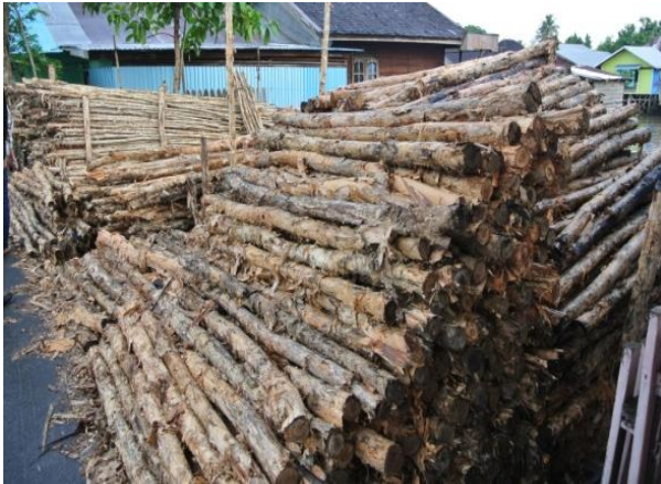
Figure 3-9. Galam , Banjarese Houses' Material (Source: Field Survey)
