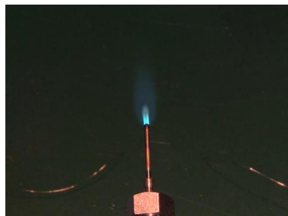
5. Stop gases supply after welding. When gases are stopped, the oxidizer valve must be closed at first to prevent back fire. Finally close the fuel valve.
