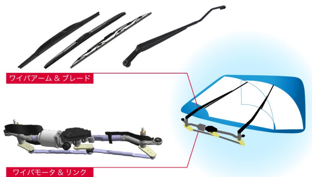
Fig. 1-1 Structure of typical wiper system (1)
