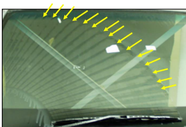
Fig. 1-6 Vibration makes caused by stick-slip motion
