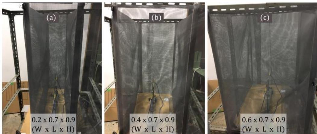
Fig. 3.4 Instantaneous photograph of various encompassments of mesh-screen for the experimental test section.
