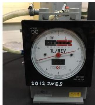
Fig. A-3.1 A typical snapshot of dry test gas meter.
