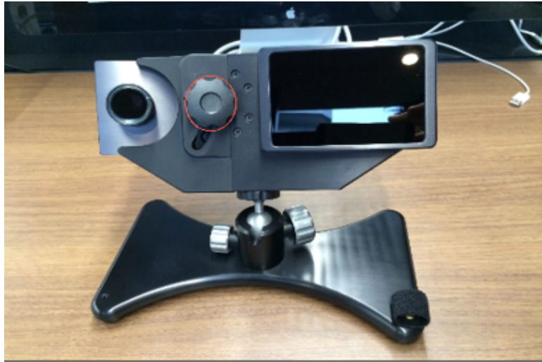
Figure 1.2: Eye-tracking device (Eyelink 1000, SR Research)
