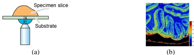
Figure 1.4. The layout of the proposed system and (b). the acoustic impedance result proposed by Hozumi et al. in 2005.
