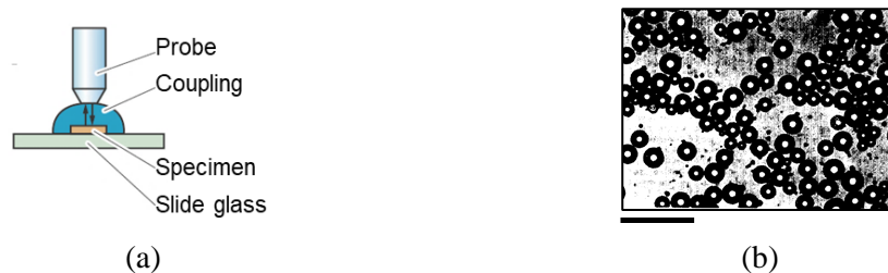
Figure 1.1. The proposed scanning acoustic microscope system and (b) the acoustic image of polystyrene particles (black bar indicates 100\ \mu\text{m} ) by Lemons et al in early 1971.
