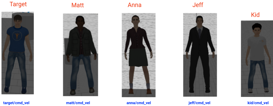
Figure 6.5: All the human models inside the dynamic environment can be controlled by publishing the linear velocity v and angular velocity \omega through specific ROS topics.
