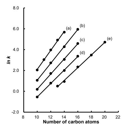
**Figure 4.3** Retentivity for normal alkanes having different carbon numbers at various column temperatures on the fibrous PI stationary phase. GC conditions; column head pressure, 100 kPa; injection mode, split; split ratio, 50:1. (a) 40°C, (b) 60°C, (c) 80°C, (d) 100°C and (e) 120°C. Other conditions are in the text.
