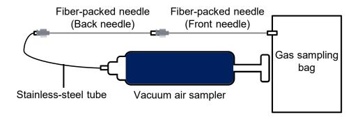
**Figure 5.5** Illustration of experimental setup for the evaluation of the extraction capacity of fiber-packed needle.
