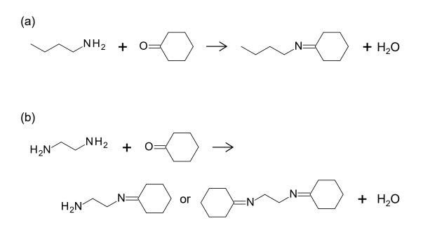
**Figure 5.7** Reaction scheme of the derivatization reaction for (a) NBA and (b) EDA with cyclohexanone.
