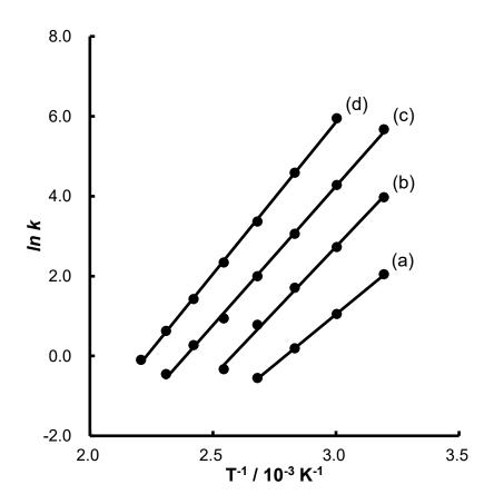
**Figure 4.4** van't Hoff plots for four alkanes on the PI stationary phase. (a) decane, (b) dodecane, (c) tetradecane and (d) hexadecane. GC conditions are the same as in Figure 4.3.
