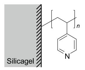
**Figure 2.2** Chemical structure of the P4VP stationary phase.
