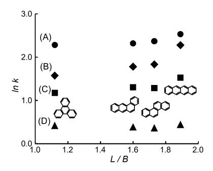
**Figure 3.3** Correlation between L/B and ln k for planar four-ring PACs on four stationary phase. (A) PBT, (B) polymeric, (C) monomeric and (D) PBS. Mobile phase: methanol/water = 90/10.
