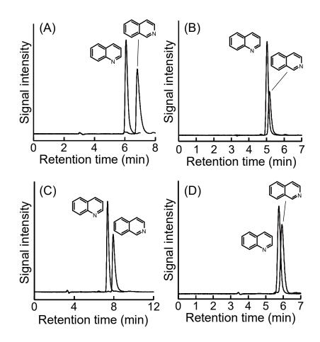
**Figure 3.6** Typical chromatograms of quinoline and isoquinoline on four stationary phases. (A) PBT, (B) monomeric, (C) polymeric and (D) PBS. Mobile phase: methanol/water = 75/25.
