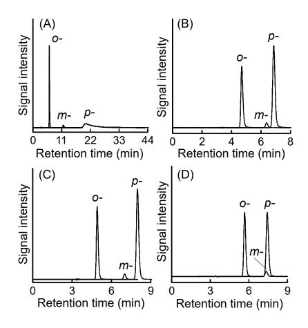
**Figure 3.5** Chromatograms for the separation of dimethyl phthalates. (A) PBT, (B) monomeric, (C) polymeric and (D) PBS. Mobile phase: methanol/water = 75/25.
