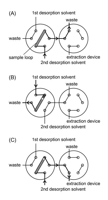
**Figure 6.7** Scheme of the sequential pumping procedure with two types of organic solvents. (A) Fill the sample loop of the injection valve with the 2nd desorption solvent, (B) switch the injection valve, and inject certain volume of 1st desorption solvent, where a small volume of air was inserted between section of the 2nd and 1st desorption solvents, (C) switch the valve again, and start the sequential pumping of two desorption solvents.
