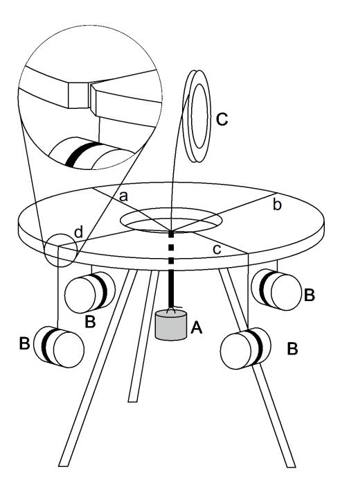
**Figure 6.2** A laboratory-made set-up for the preparation of braided fiber. (A) Center weight; (B) bobbins; (C) stainless-steel wire.
