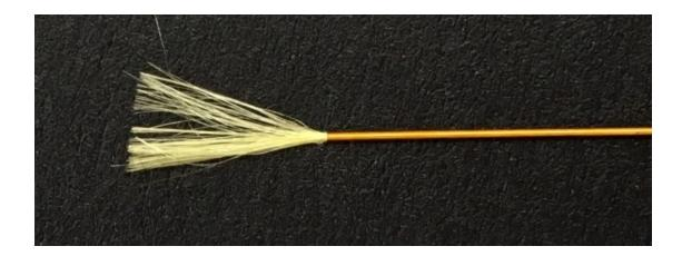
**Figure 4.2** Typical photograph of PI fiber-packed capillary column.
