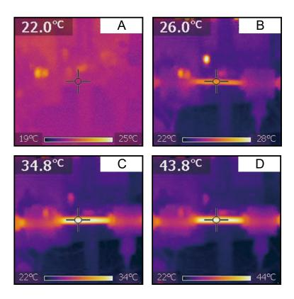
**Figure 6.8** Thermographic observation of the surface temperature of the extraction capillary during a resistive heating process. Applied voltage: (A) 0V, (B) 1V, (C), 2V and (D) 3V. Other conditions are in the text.
