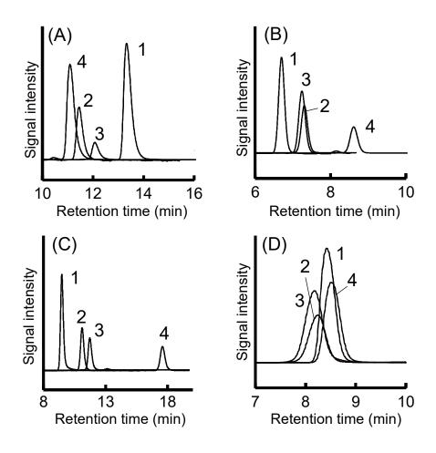
**Figure 2.4** Typical chromatograms of planar four-rings PACs on (A) P4VP, (B) monomeric ODS, (C) polymeric ODS and (D) PBS phases. Analyte: 1, triphenylene (L/B = 1.12); 2, benz[*a*]anthracene (L/B = 1.58); 3, chrysene (L/B = 1.72); and 4, naphthacene (L/B = 1.89). Mobile phase: methanol/water = 90/10.
