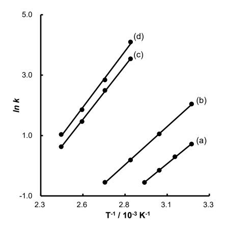
**Figure 4.5** Typical van't Hoff plots for alkanes and alcohols obtained on the PI stationary phase. (a) nonane, (b) decane, (c) 1-nonanol and (d) 1-decanol. GC conditions are the same as in Figure 4.3.
