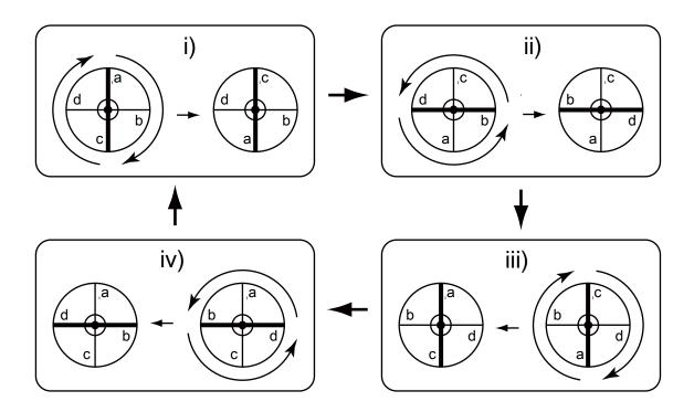
**Figure 6.3** Preparation of braid-type extraction medium. Bobbin positions (a)-(d) correspond that in Figure 6.2. First, i) a pair of bundles placed at the opposite of the circular plate (a and c) were simultaneously moved clockwise 180°, and then, ii) another pair of bundles (b and d) were also simultaneously moved counterclockwise 180°. This two-step process was repeated once more as shown in iii) and iv), to return to the original configuration i).
