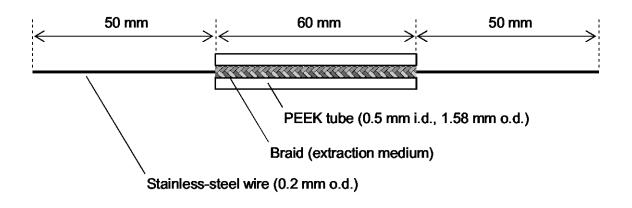
**Figure 6.5** Schematic of the braid-packed extraction capillary with a stainless-steel wire therein.
