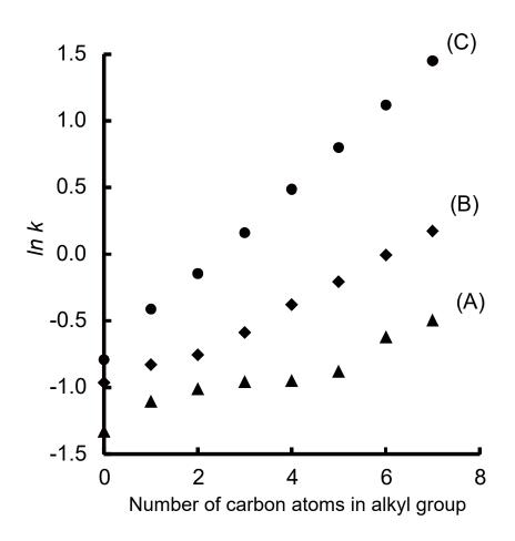
**Figure 2.5** Relationship between the number of carbon atoms in alkyl chain and *ln k* of alkylbenzenes on three stationary phases. (A) P4VP, (B) PBS and (C) monomeric ODS. Mobile phase: (A) methanol/water = 70/30, (B) and (C) methanol/water = 90/10.
