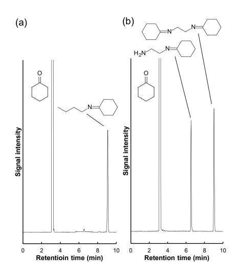
**Figure 5.8** Chromatograms for the separation of (a) NBA derivative and (b) EDA derivative using the fiber-packed needle with cyclohexanone as the derivatization reagent. Extraction conditions: flow-rate, 2.5 mL/min; sampling volume, 50 mL; desorption temperature, 270°C; analyte, (a) NBA (200 ppm) in  $N_2$  and (b) EDA (200 ppm) in  $N_2$ . Other conditions are the same as in Figure 5.3.
