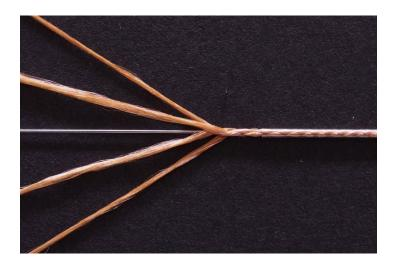
**Figure 6.4** Typical photograph of a braided fiber prepared in this work.
