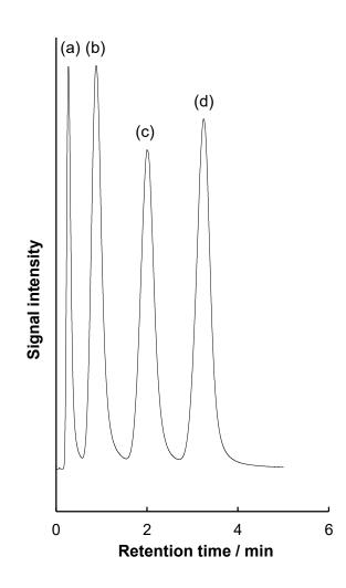
**Figure 4.7** Chromatograms for the separation of a homologous alkane mixture. Conditions: temperature program, 50°C to 150°C at the rate of 20°C/min. Peaks: (a) decane; (b) dodecane; (c) tetradecane and (d) hexadecane. Other conditions are the same as in Figure 4.3.
