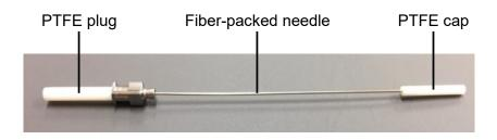
**Figure 5.4** Photograph of fiber-packed needle sealed using PTFE plug and cap.
