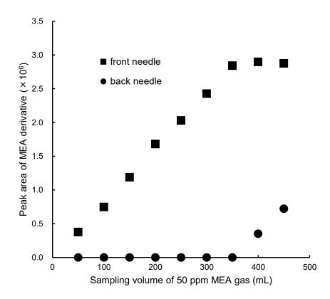
Figure 5.6 Extraction capacity of the needle extraction device for MEA. Extraction conditions: flow-rate, 2.5 mL/min; sampling volume, 50 to 450 mL; desorption temperature, 270°C; analyte, MEA (50 ppm) in  $N_2$ . Other conditions are the same as in Figure 5.3.
