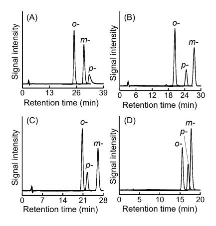
**Figure 3.4** Chromatograms for the separation of dibromobenzenes. (A) PBT, (B) monomeric, (C) polymeric and (D) PBS. Mobile phase: methanol/water = 70/30.
