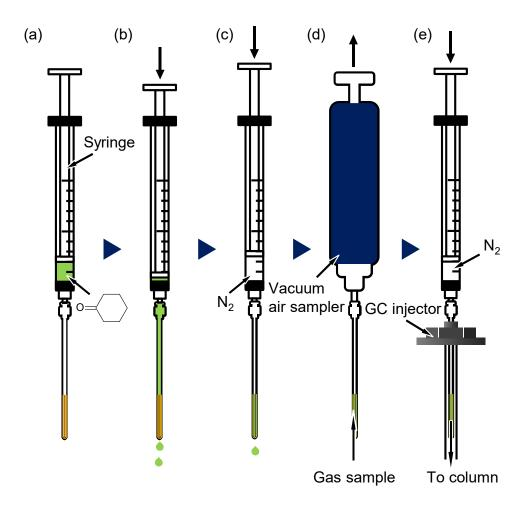
**Figure 5.2** Sample preparation procedure with cyclohexanone as the derivatization reagent for volatile amines in air samples.
