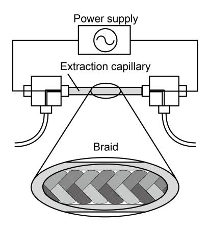
**Figure 6.6** Illustration of the miniaturized SPE device connected with an electric power supply developed in this work.
