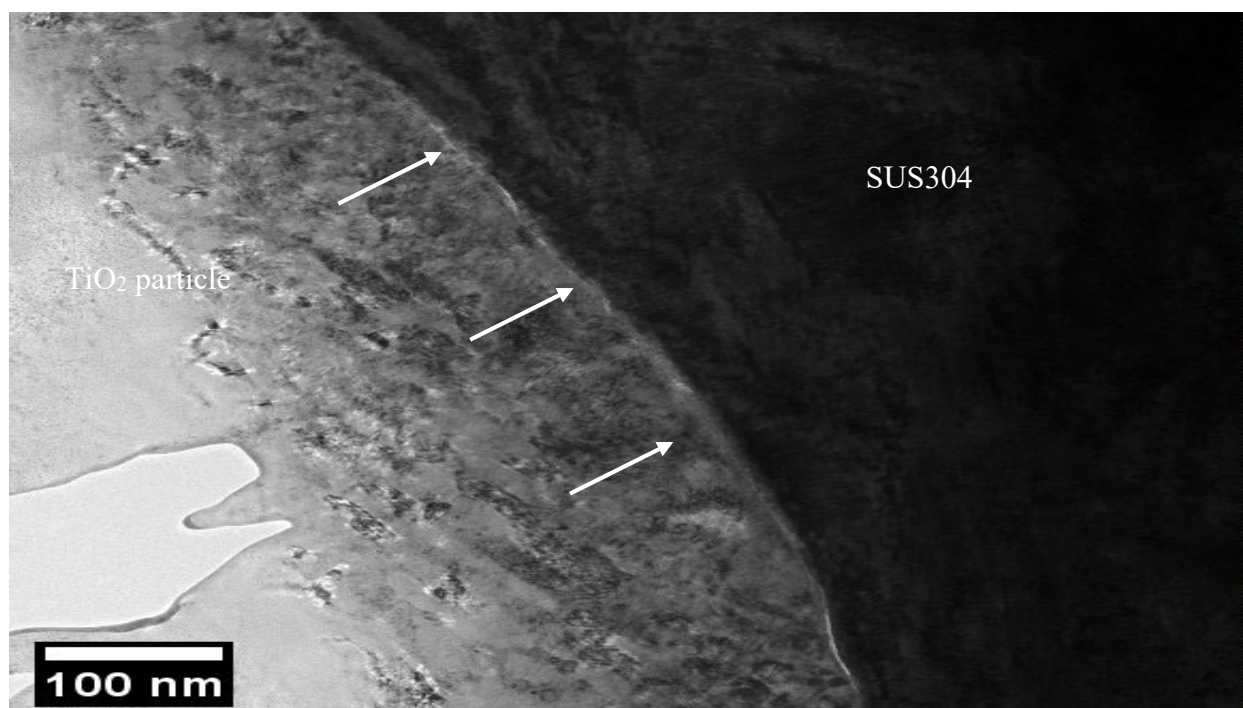
Figure 4.21: STEM of the TiO 2 / 1000°C annealed SUS304 at the interlayer area.
