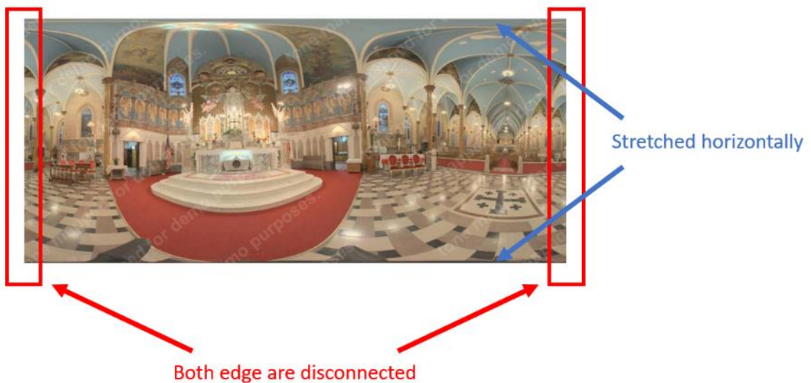
Figure 5.3: Planar light probes lose accurate spatial structure. When a light probe of a spherical surface is transformed into a two-dimensional image for Fourier transformation, the left and right edge that should be connected become disconnected. Also, the frequency response changes as the image is stretched closer to the top and bottom edges.
