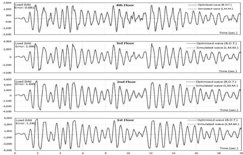
Figure 21: Model Building, Story shear history.
