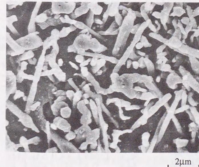
Fig.2-5 SEM image of typical whisker distribution in the as-fabricated composite.
