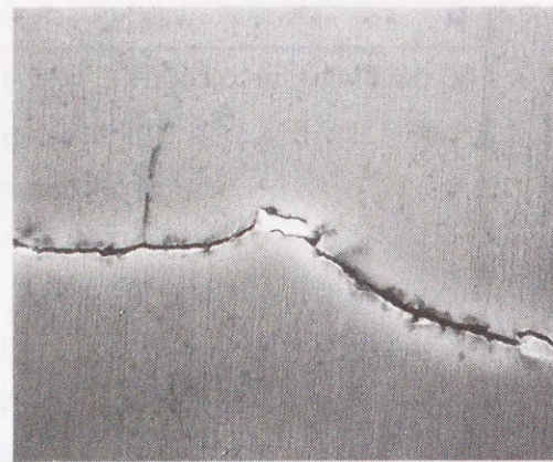
(a) Crack initiation from IMC particle
