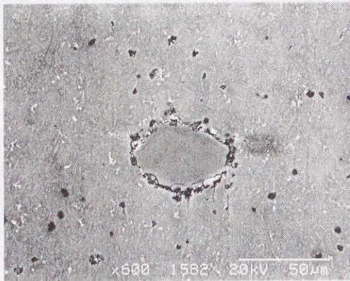
(c) Crack initiation from coarse particle
