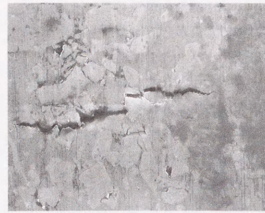
(b) Crack initiation from clustering whisker
